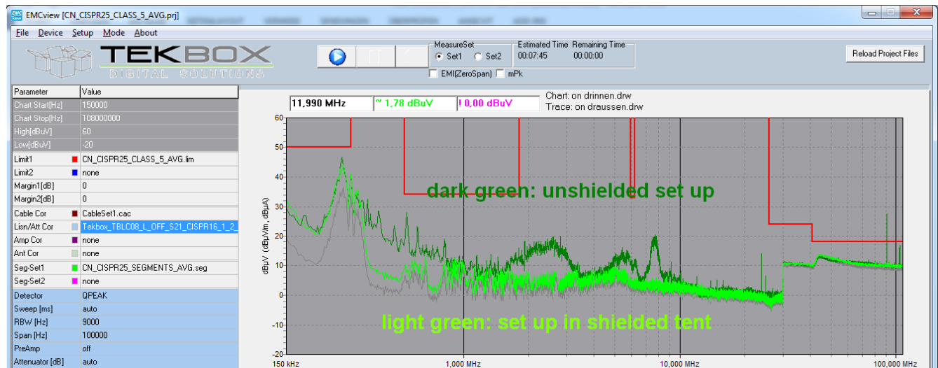
Picture 6: CISPR 25 conducted noise measurement; DUT powered
