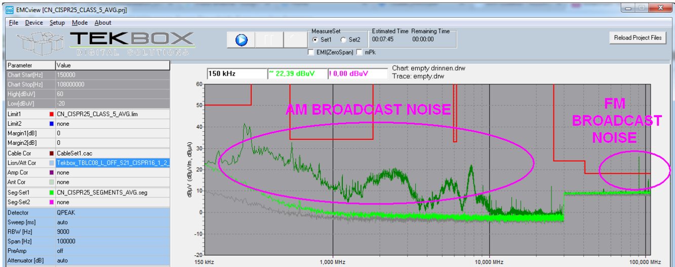
Picture 5: CISPR 25 conducted noise measurement; DUT not powered
